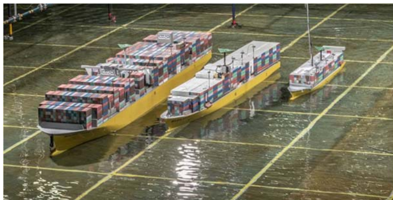
Vessels tested at MARIN: ULCS, Panamax and Feeder
